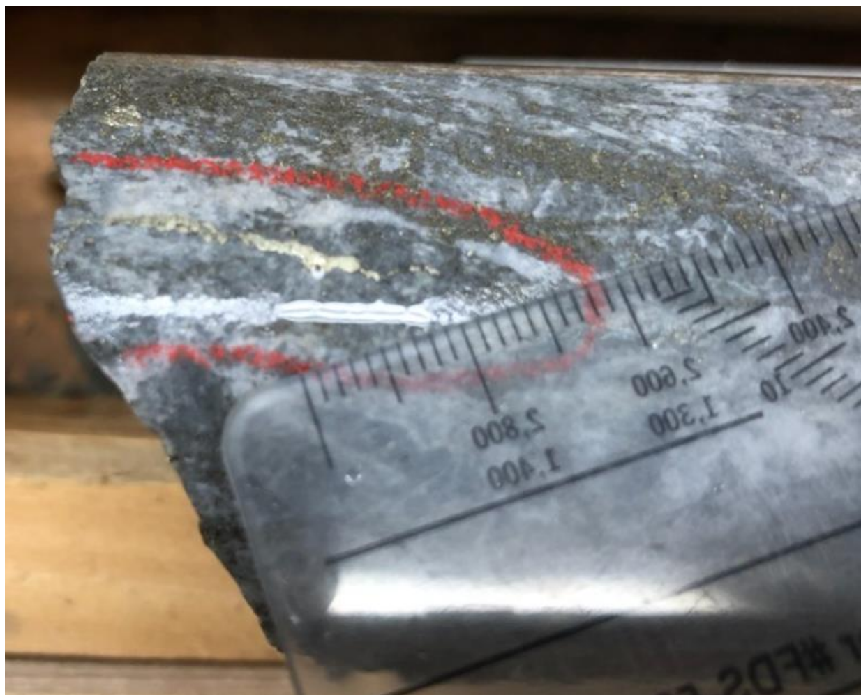
Figure 3 Image showing a 1.5cm particle of native gold in drill core from hole P20-2183.
