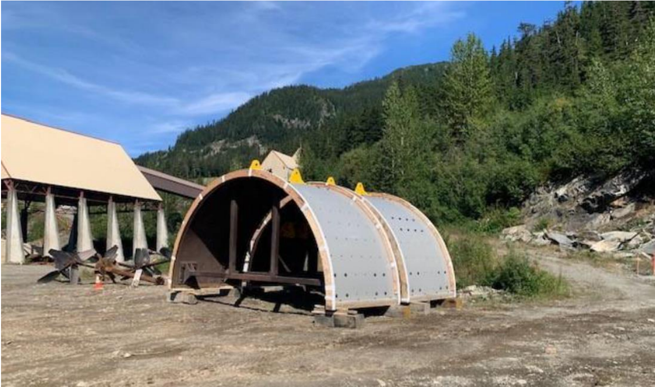
Figure 4 SAG mill shell delivered.
