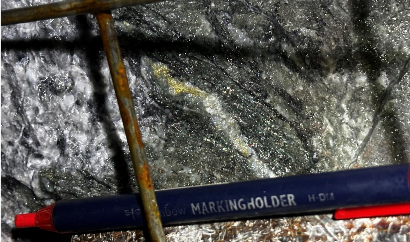
Figure 1 – Visible gold in quartz vein found in ore drive 6 at Big Missouri
