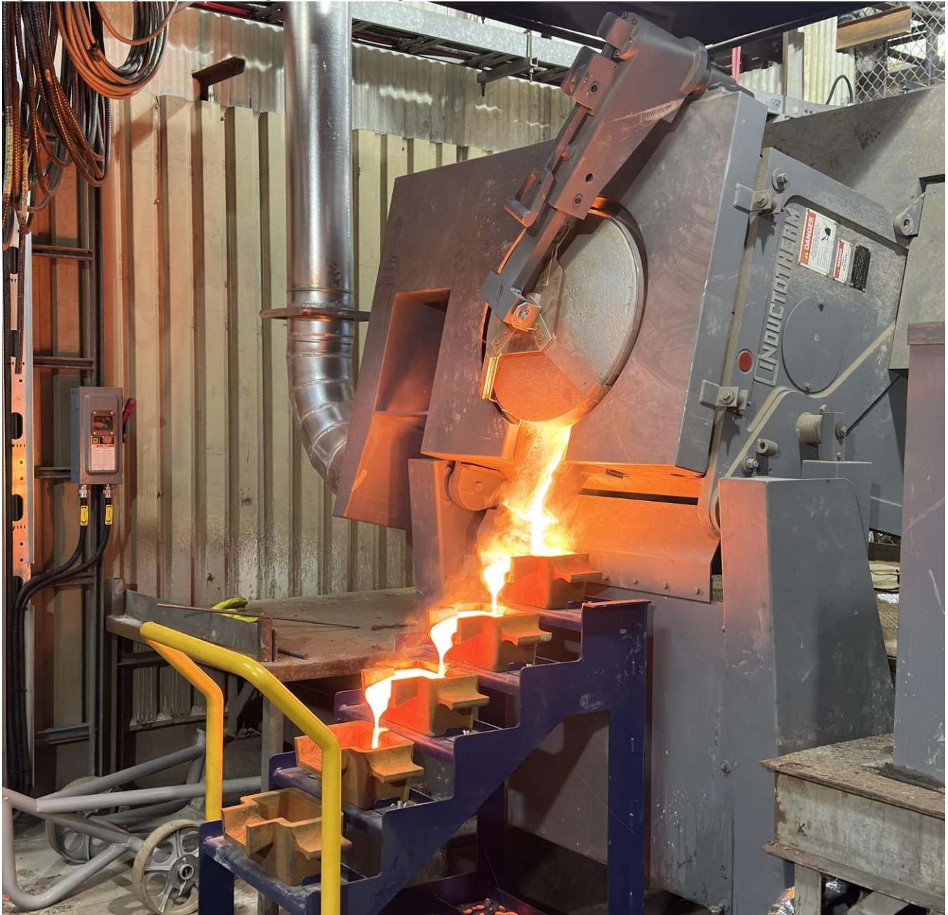
Figure 1 – First gold pour during commissioning at PGP
